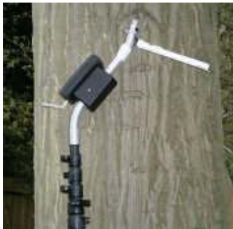
168. The nest camera. The viewing head on the right goes into the nest hole. The black box contains the batteries and a small radio link to transmit the pictures to the portable video recorder. The telescopic carbon fibre poles allow high nests to be inspected. Ken Smith
